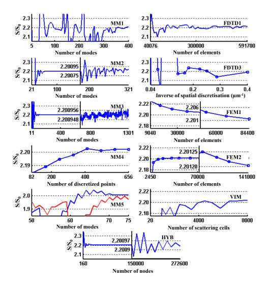
FIG. 4 Absolute convergence performance of the different methods as a function of the parameter N related to the sampling accuracy of the method, starting from an arbitrary  $N_{\min}$  value up to a  $N_{\max}$  value obtained before memory or time limitations. Two curves corresponding to two different PML implementations are provided for MM5.
