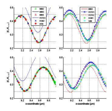
FIG. 7 Comparison between the different methods for the normalized total field  $|E_x/E_{x,inc}|$  as function of the x-coordinate at  $y = 0^+$ . Top: small x values. Bottom: large x values. The repartition of the method results between the left and right sides of the figure is arbitrary. This choice is simply motivated by clarity reasons.
