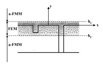
FIG. 2 Sketch of the zone handled with FEM and a-FMM in the HYB method.
