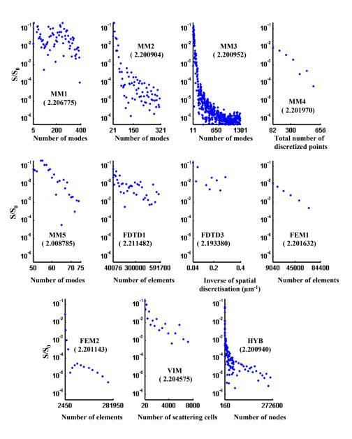
FIG. 5 Convergence performance of the different methods as a function of the parameter N starting from one arbitrary  $N_{\min}$  value up to a  $N_{\max}$  value obtained before memory or time limitations. The error is defined as  $|[S/S_0(N)]/[S/S_0(N_{\max})] - 1|$ , and the number in parenthesis located below the method acronym represents  $S/S_0(N_{\max})$ .
