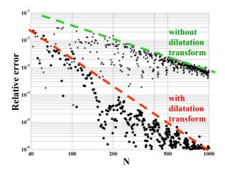
FIG. 10 Impact of the dilatation transform at the slit and groove boundaries on the performance of the MM3 for d = 500 nm. Stars and dots are respectively obtained without and with the transform. N represents the total number of Fourier harmonics retained in the calculation. The relative error is defined as  $|S/S_0 - T_0|/T_0$ , with  $T_0 = 2.200952$  being the best extrapolated value for  $S/S_0$ .
