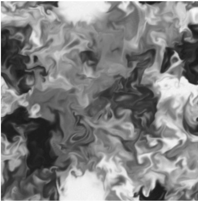
FIG. 3. A view of the scalar field for a 256 3 DNS. A recent injection can be seen, appearing as a white homogeneous zone.
