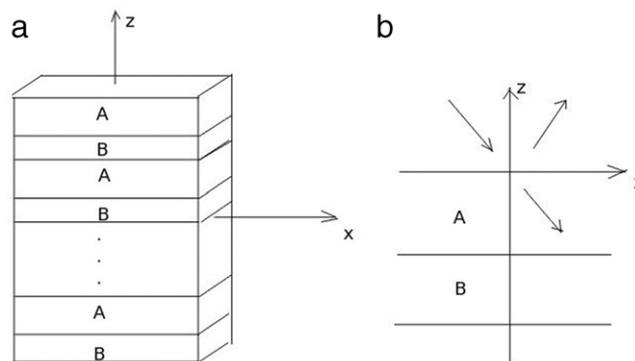
Fig. 1. As in [1], we study a stack of alternating layers. Layer A has an optical index of 1 ( $\varepsilon_1 = 1$ ) and has a thickness of  $a = 0.75$  in arbitrary units. Layers of type B present an optical index of 2.3 ( $\varepsilon_2 = 5.29$ ) and are  $b = 0.25$  thick. The finite structure contains 10 periods. The wavelength is of 1.0744 to get a negative group velocity.
