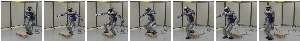
Fig. 12. The HRP-2 over crossing a 15 cm platform: the HRP-2 takes steps the platform with one foot and over-cross it with the other.
