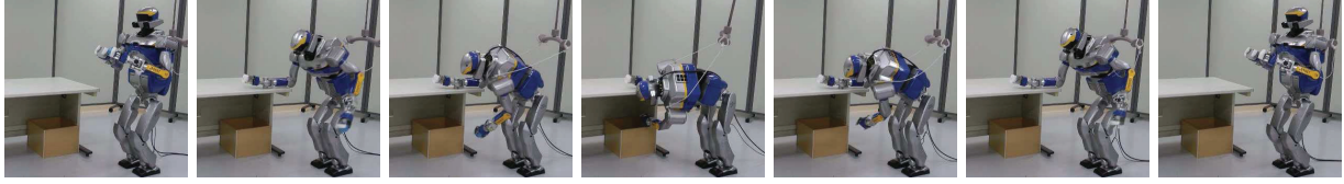
Fig. 10. With the right arm, the HRP-2 robot takes an additional support on the desk, which allows it to stably lean and put a ball into the trash box located under the desk.
