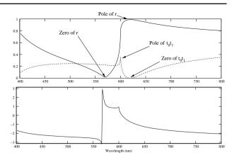
**Figure 2.** Typical example of |r| (top, solid line),  $|t_0 t_1|$  (top, dotted line) and  $\phi$  (bottom, solid line) for the semi-infinite structure with d = 600 nm and a = 100 nm.
