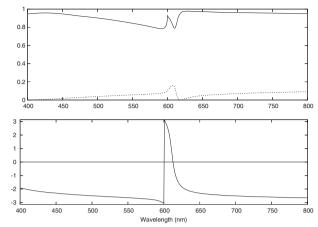
**Figure 5.** Modulus of *r* (top, solid line),  $|t_0t_1|$  (top, dotted line) and phase of *r* (bottom, solid line) for the semi-infinite structure with d = 600 nm and a = 10 nm. The pole of  $t_0t_1$  moves towards the pole of *r*. It is located at  $\lambda = 608$  nm.
