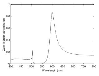
**Figure 8.** Zeroth-order transmission of a slit array with d = 504.9 nm, a = 115.7 nm and h = 127.9 nm (solid line) and the single-mode approximation result (dashed line). The peak at  $\lambda = 504.9$  nm is due to the excitation of the horizontal resonance on both sides of the structure. The parameters of this structure have been found using optimization, so that the 0 resonance has a maximum @600 nm.
