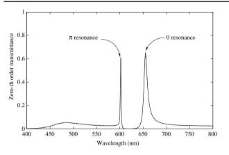
**Figure 9.** Zeroth-order transmission of a slit array with d = 600 nm, a = 45.5 nm and h = 120 nm (solid line) and the single-mode approximation result (dashed line). The 0 and the  $\pi$  resonance can be seen on the same spectrum.
