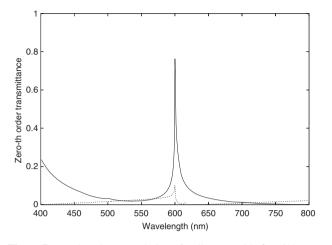
**Figure 7.** Zeroth-order transmission of a slit array with d = 600 nm, a = 51.37 nm and h = 33.89 nm (solid line) and the single-mode approximation result (dashed line). The one-mode model is clearly inaccurate for these parameters: the enhanced transmission is due to the excitation of a horizontal resonance. The geometrical parameters have been obtained using optimization (see hereafter).
