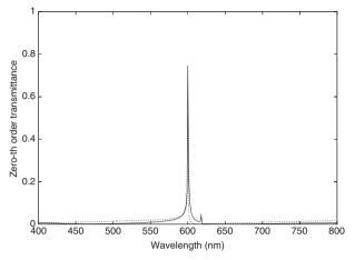
**Figure 10.** Zeroth-order transmission of a slit array with d = 600 nm, a = 45.5 nm and h = 60.5 nm (solid line) and the single-mode approximation result (dashed line). The parameters of this structure have been found by optimization, so that the  $\pi$  resonance presents a maximum @600 nm.
