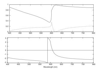
**Figure 4.** Modulus of *r* (top, solid line),  $|t_0t_1|$  (top, dotted line) and phase of *r* (bottom, solid line) for the semi-infinite structure with d = 600 nm and a = 40 nm. The zero of *r* moves towards the left, and the quick variation of the phase follows. The poles of *r* and  $t_0t_1$  do not move.
